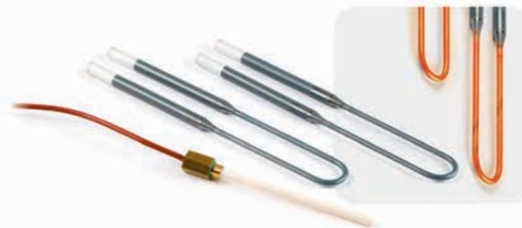
High-quality molybdenum disilicide heating elements reach a maximum end temperature of 1.650°C. Unlike silicon carbide heating systems, heaters of this type are far enough away from their maximum performance limit of approx. 1.800°C. Thanks to this property they attain a significantly longer service life. Each of the four heating elements can be individually replaced in case of damage – an „en bloc“ replacement is unnecessary.
