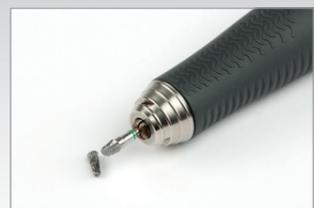
**Milling bit broken**
