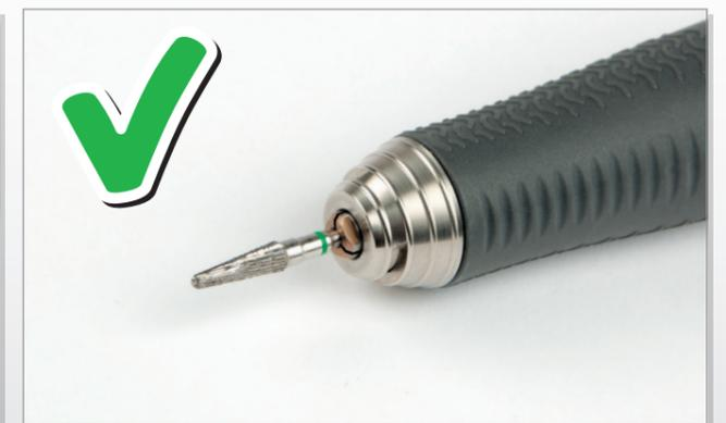
Milling bit correctly clamped.
