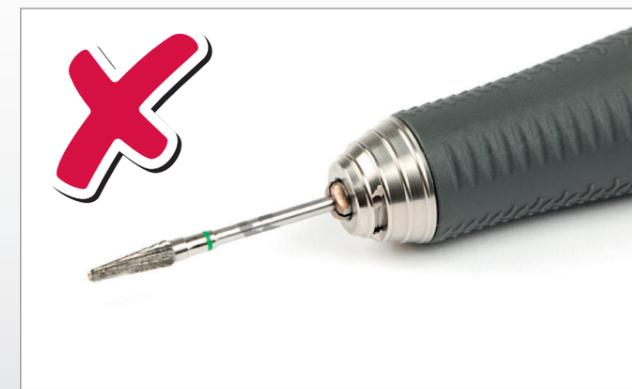
Milling bit is not inserted deep enough into the collet chuck.
