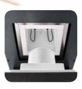
High-quality molybdenum disilicide heating elements reach a maximum end temperature of 1.650°C. Unlike silicon carbide heating systems, heaters of this type are far enough away from their maximum performance limit of approx. 1.800°C. Thanks to this property they attain a significantly longer service life. Each of the four heating elements can be individually replaced in case of damage – an "en bloc" replacement is unnecessary.
