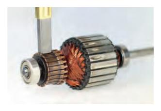
Motor after 1,000 hours with conventional control; the collector is heavily worn.
