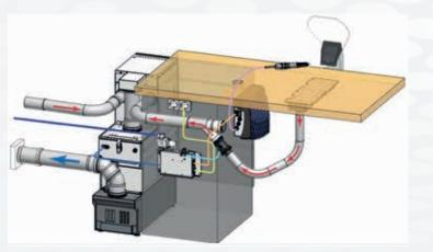
In practices or small laboratories with one or two technicians, dust can thus be extracted from the entire equipment space or work station area with one **Z2**. Use in alternative operation is particularly convenient. As long as only one suction station is in operation, the suction level can be selected as with a single-station suction system and can be individually saved for each work station.
